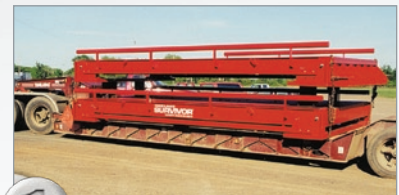
1 Self contained deck modules.
